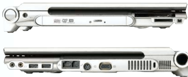
Top: The Mediastar features a memory card reader, DVD burner and a Firewire socket
